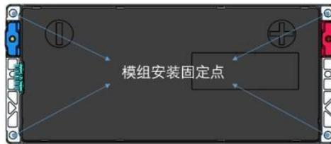
Figure 4 102Ah 1P6S Schematic diagram of fixed point for battery module installation
